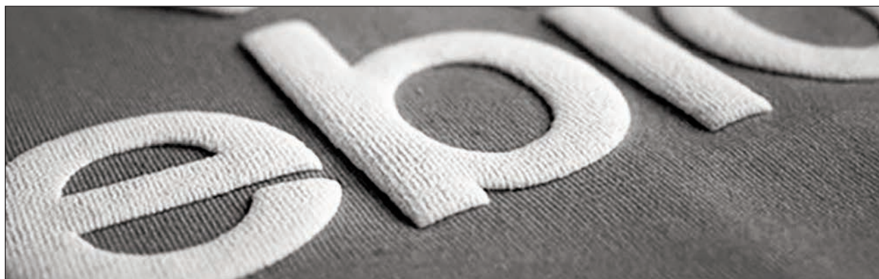
Fig. 1. Screen printing with puff effect
